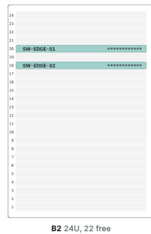
Figure 73. The Racks page as printed: rack elevations for a wall or a work order.
